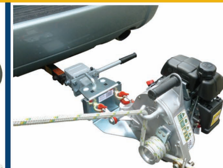
With Heck-Pack (PCA-1266) & Heck-Pack adaptor (PCA-1265) (for 50 mm towing ball)
