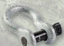
SHACKLES PCA-1279 - 13 mm (1/2") - Working load limit: 2 tons. PCA-1277 - 16 mm (5/8") - Working load limit: 3-1/4 tons. PCA-1278 - 20 mm (3/4") - Working load limit: 4-3/4 tons.
