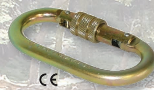
PCA-1276 Steel oval locking carabiner. 2550 kg (5500 lb) MBS.
