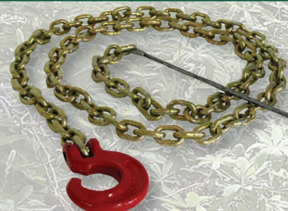
PCA-1295 Choker chain 6 mm x 2.1 m (1/4" x 7') with C-Hook and steel rod. Weight: 2.8 kg (6 lb). 5700 kg (12 600 lb) MBS
