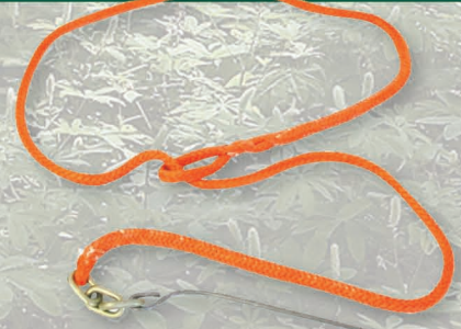
PCA-1372 HPPE rope choker 9.5 mm x 2.1 m (3/8" x 7') with steel rod. Weight: 350 g (12 oz) 7100 kg (15 500 lb) MBS.
