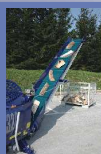
Discharge conveyor 4 m (standard equipment): two stage telescope with automatic hydraulic belt straining. Continuous speed control of the conveyor belt.
