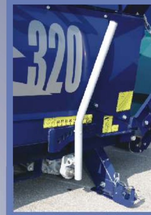
The height of the splitting wedge is adjusted with the holder to best fit the size of the cut log.
