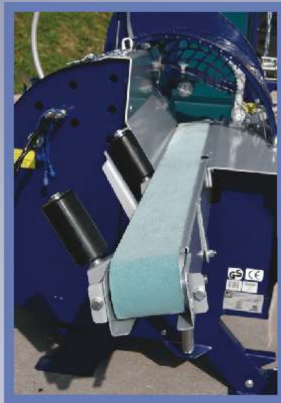
The foldable infeed conveyor (2 m) enables the forwarding of long and heavy logs
